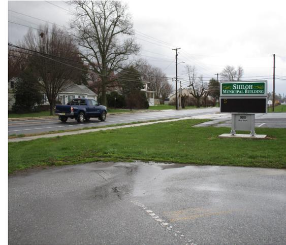
A rain garden can be installed behind the sign to capture runoff from the roof. At the east side of the building, cisterns can be installed to store stormwater runoff from the roof to be reused for multiple purposes such as washing vehicles. A preliminary soil assessment suggests that the soils have suitable drainage characteristics for green infrastructure.
