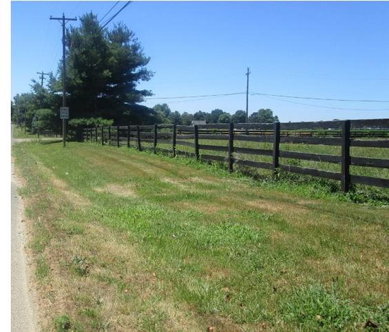
Bioswales can be installed along the fence pictured above to capture stormwater runoff from the road. The turfgrass areas alongside the road are eroding due to the flow of the runoff. These areas are also at a lower depth than that of the road, which would allow the stormwater to flow into the bioswales. A preliminary soil assessment suggests that the soils have suitable drainage characteristics for green infrastructure.
