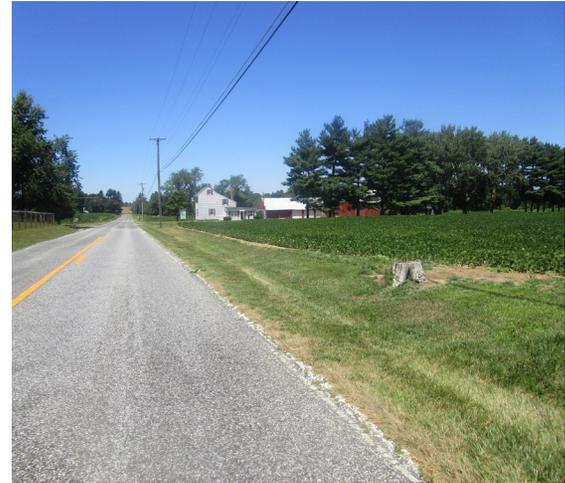
The turfgrass area north of the driveway alongside the road can be converted to a bioswale to capture stormwater runoff from the road. Additional benefits include enhancing the aesthetic of the area and providing a habitat for wildlife. A preliminary soil assessment suggests that the soils have suitable drainage characteristics for green infrastructure.
