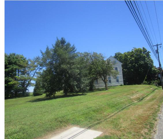
A bioswale can be installed in the area stretching from the end of the sidewalk to the first telephone pole. The area is trench-like, with a lower depth alongside the road that rises moving inward towards the field. A preliminary soil assessment suggests that the soils have suitable drainage characteristics for green infrastructure.
