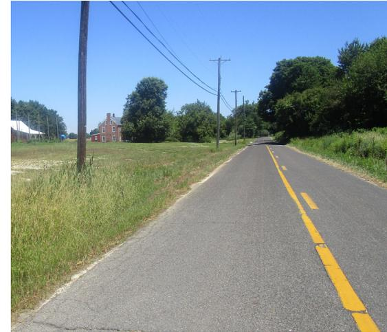
The turfgrass area alongside the road west of the building can be converted into a bioswale. Currently, the soil along the roadside is eroding and puddles with stormwater runoff. This problem can be solved with the creation of a bioswale. A preliminary soil assessment suggests that more soil testing would be required before determining the soil's suitability for green infrastructure.
