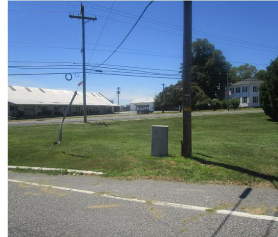
The turfgrass area is at a lower elevation than the road; curb cuts can be made to allow stormwater to flow into a rain garden. This system will manage stormwater runoff from the road, enhance the aesthetic of the area, and create a habitat for wildlife. A preliminary soil assessment suggests that the soils have suitable drainage characteristics for green infrastructure.
